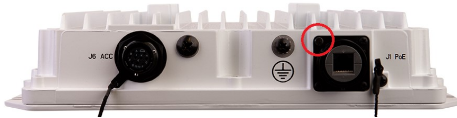
Figure 5 – Tamper-Evident Pin Location for RF-7800W
