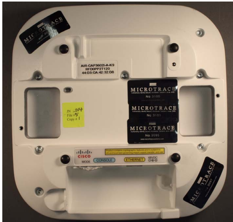
Figure 4 Seals Covering Screws On Module Enclosure and Module Connector Slot
