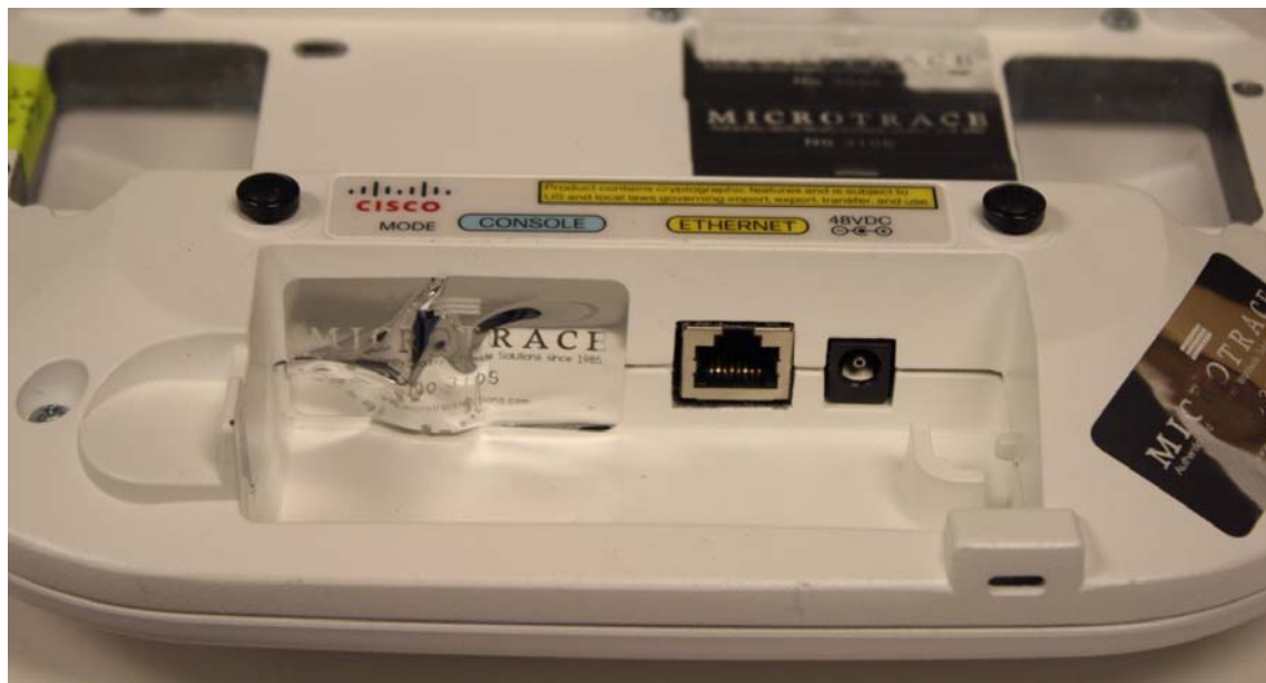
Figure 3 Seal Covering Console Port and Mode Button
