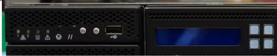
Figure 2-6 SV3800/SV3800B/SV3800B-20 Front Panel Controls and Display
