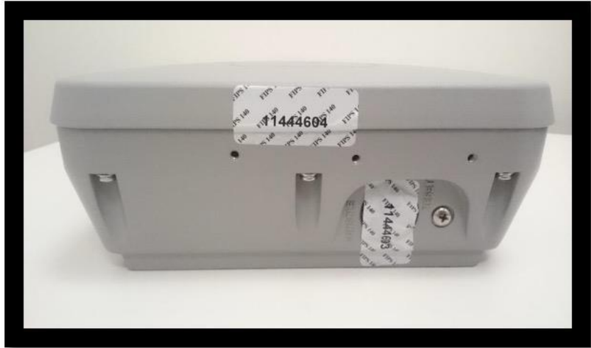
Figure 45: TEL Placement 3 and 4
