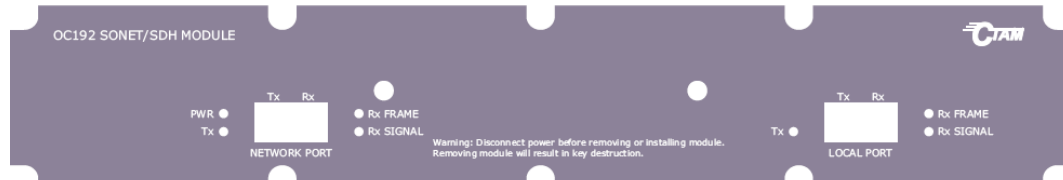
Figure 8 - A5213, A5214 OC-192/STM64 – SONET/SDH Rear Interface Label
