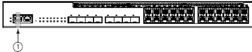
Figure 15 Front view of a Brocade ICX 6610-24F device with security seals
