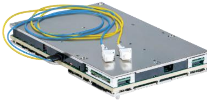
Figure 1: Acacia AC1200 pluggable encryptor unit
