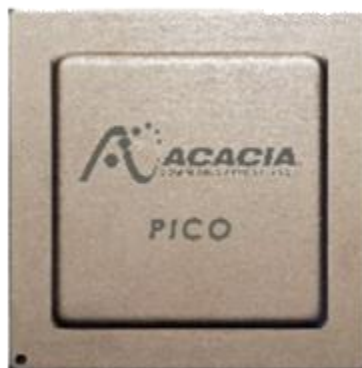
Figure 2: Acacia Pico DSP (housed inside AC1200)
