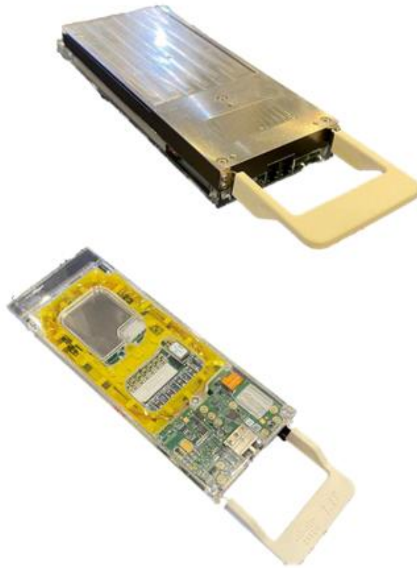
Figure 3: Acacia AX1200 (with Jannu DSP) physical perimeter
