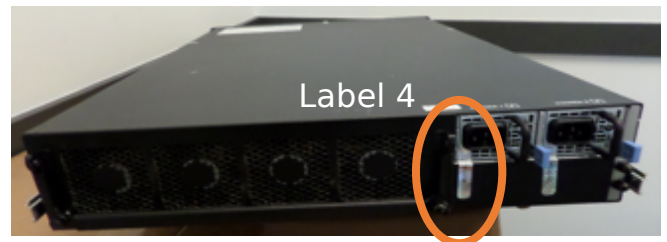
Figure 13 - Tamper labels on BIG-IP i10800, BIG-IP i10600 and BIG-IP i11600-DS, BIG-IP i11800-DS (4 tamper labels shown)
