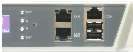
Figure 12 – RJ45 Ethernet, Console and USB close-up
