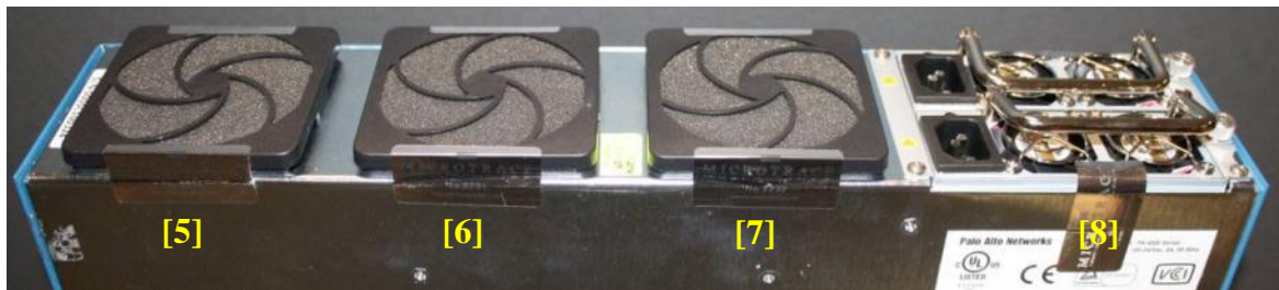
Figure 44 - PA-4000 Series Rear Side Tamper Seal Placement – From Underside (4)
