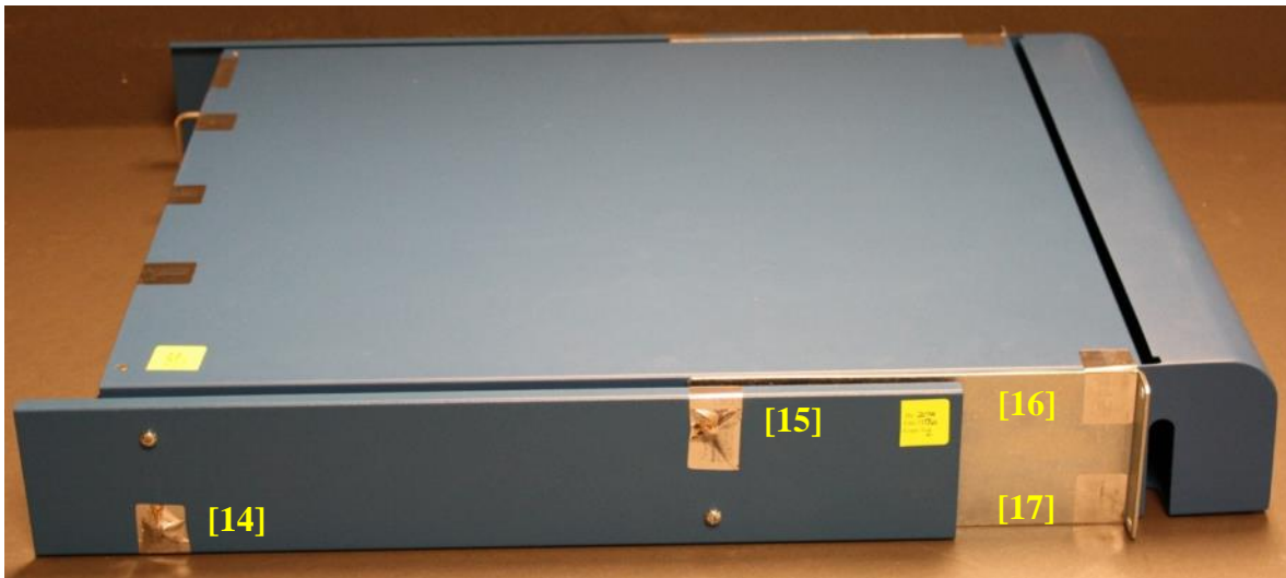
Figure 49 - PA-5000 Series Left Side Tamper Seal Placement (4)
