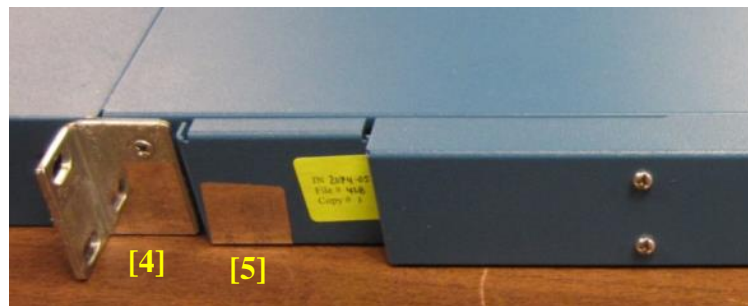
Figure 41 - PA-3000 Series Tamper Seal Placement (2)
