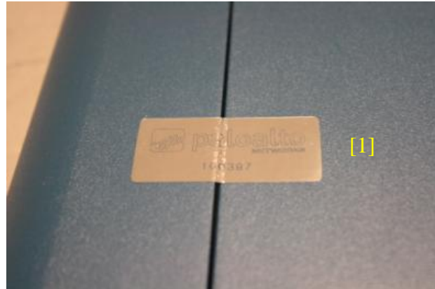
Figure 32 - PA-500 Front Tamper Seal Placement (1)
