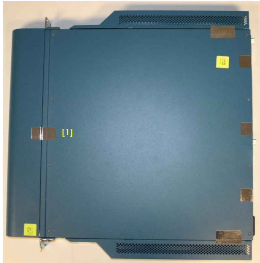
Figure 36 - PA-2000 Series Front Tamper Seal Placement (1)
