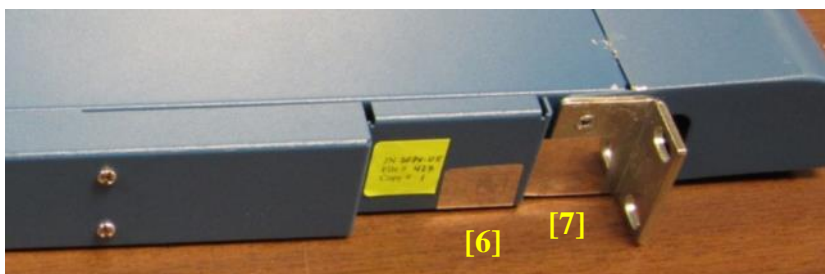
Figure 42 - PA-3000 Series Tamper Seal Placement (2)
