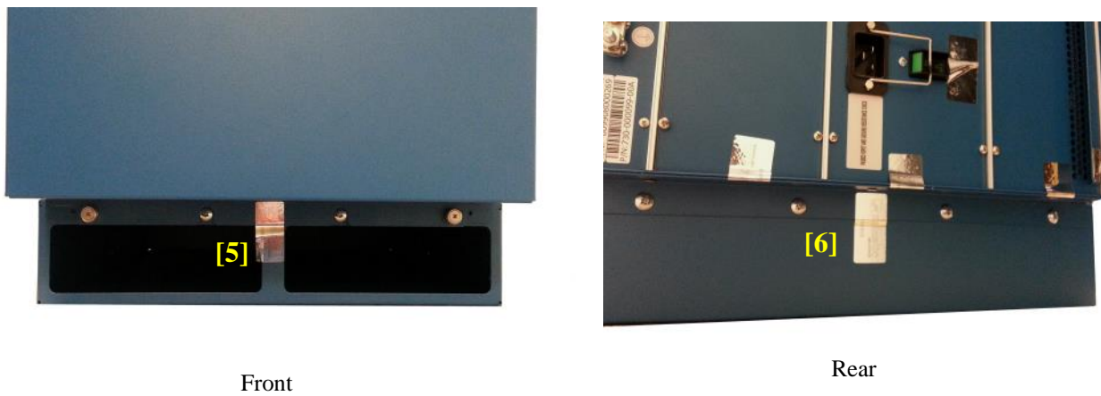
Figure 51 - PA-7050 Tamper Seal Placement for Bottom Plenum (5-6)
