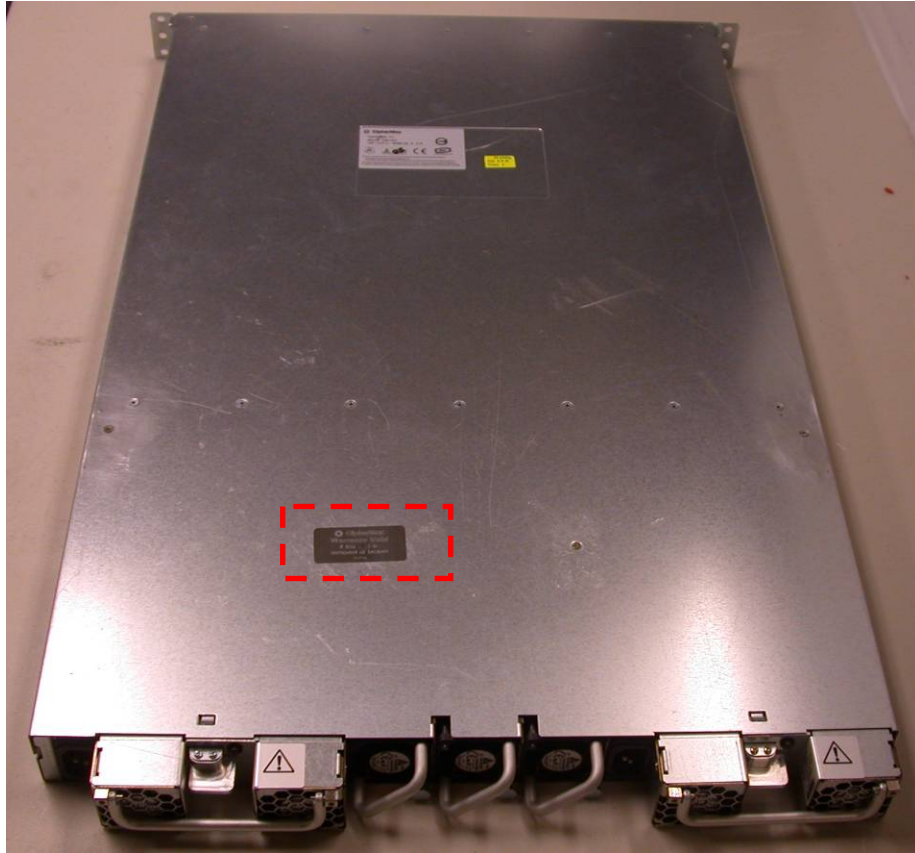
Figure 2 – CM140T Tamper-Evident Seal Placement (shown in the red rectangle above)
