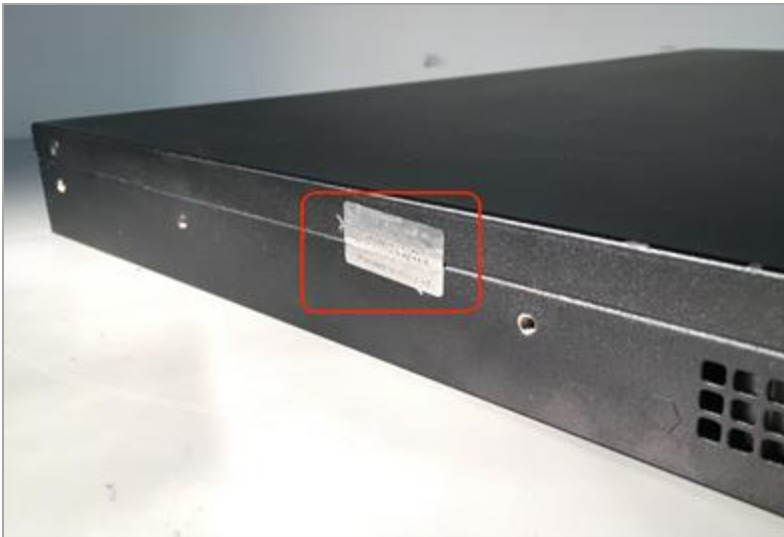
Figure 2 - CSa 1000 Tamper Seal #1 - Chassis Seam
