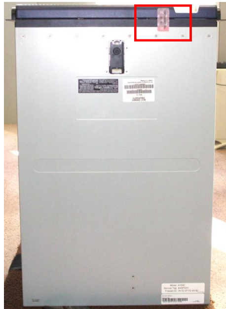
Figure 6 – Tamper-Evident Seal Application Position (Front Bezel)
