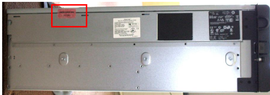
Figure 7 – Tamper-Evident Seal Application Position (Top Cover)
