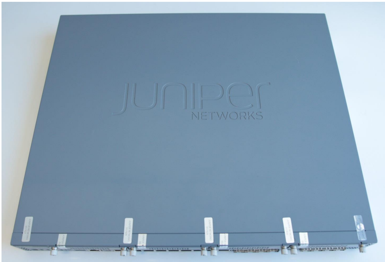
Figure 5 - SRX345 Tamper-Evident Seal Placement (Top Cover, Nine (9) Seals)
