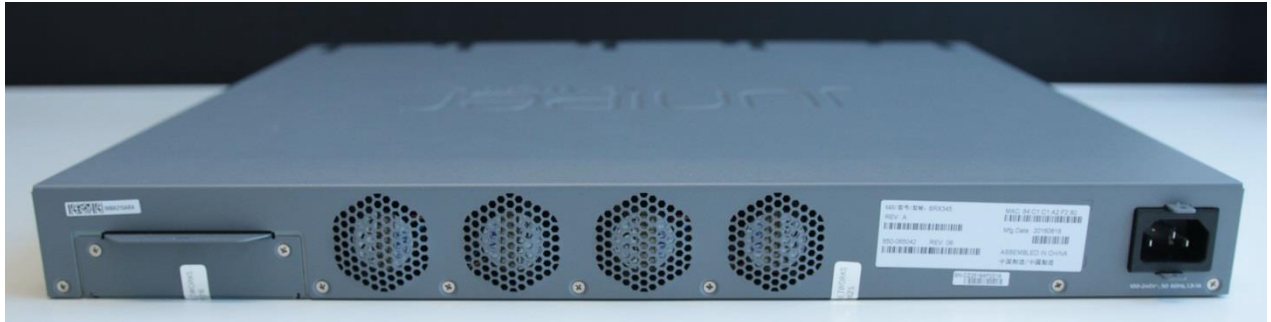
Figure 6 - SRX 345 Tamper-Evident Seal Placement (Rear Panel, Two (2) Seals)
