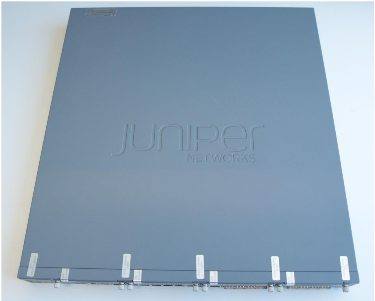
Figure 9 - SRX345-DUAL-AC Tamper-Evident Seal Placement (Top Cover, Nine (9) Seals)
