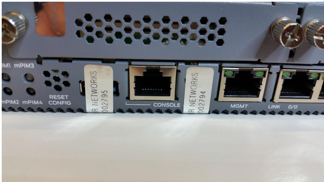
Figure 8 - SRX345 Tamper-Evident Seal Placement (USB Ports, Two (2) Seals)
