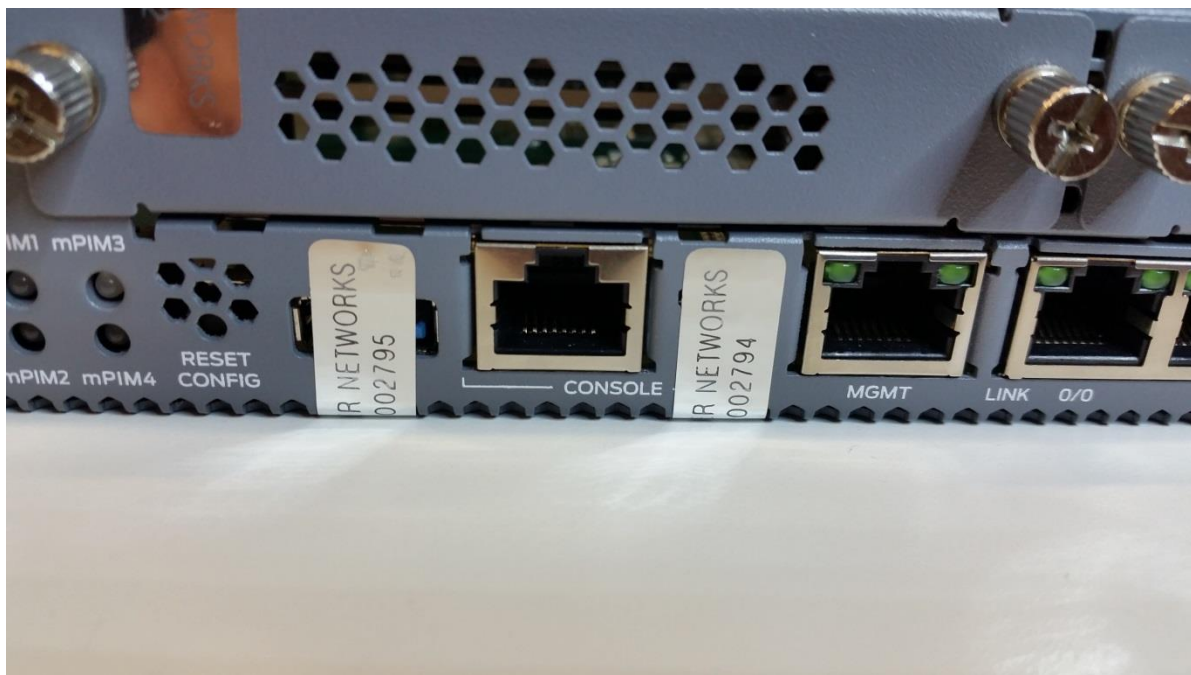
Figure 11 - SRX345-DUAL-AC Tamper-Evident Seal Placement (USB Ports, Two (2) Seals)
