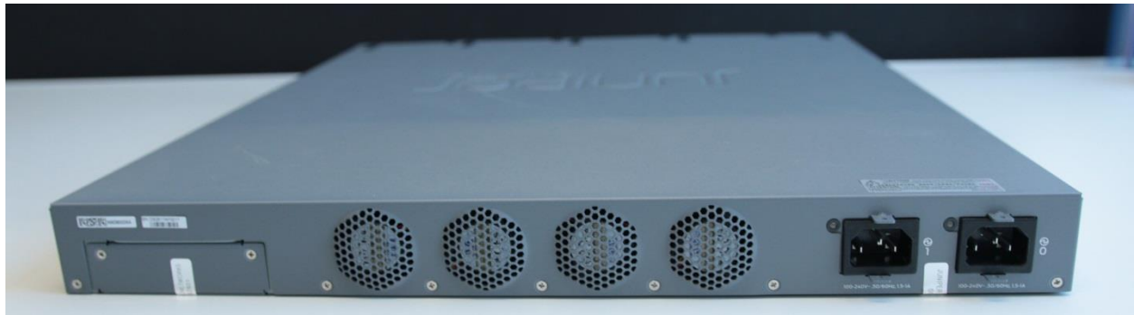
Figure 10 – SRX345-DUAL-AC Tamper-Evident Seal Placement (Rear Panel, Two (2) Seals)
