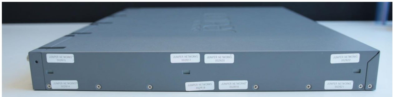
Figure 7 - SRX345 Tamper-Evident Seal Placement (Side Panels, Eight on each side – Sixteen (16) Seals)
