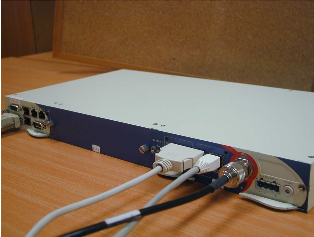
Figure 2. FibeAir 1500P™ Secure Basic Indoor Unit with Interface Ports Connected: Radio, Fast Ethernet and 8xT1;
