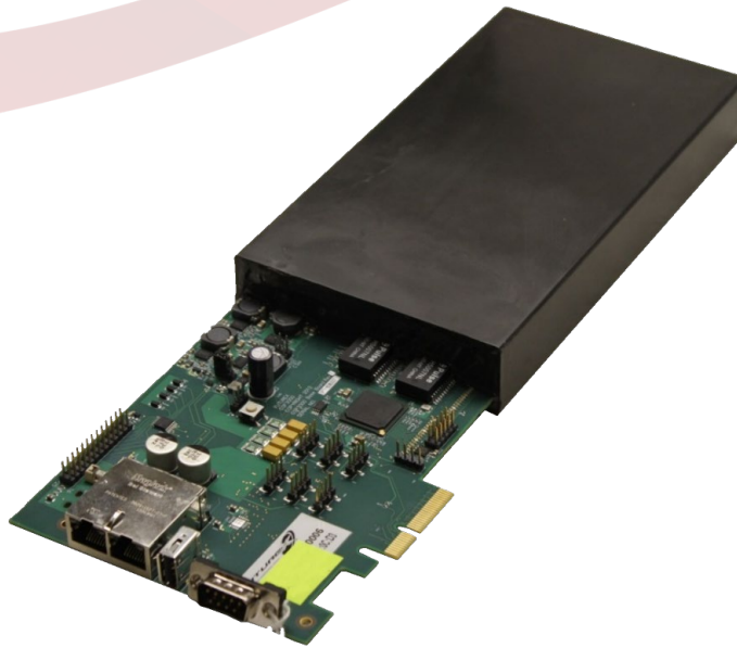
Figure 3 – GSP3000 with its Tamper Potting Intact
