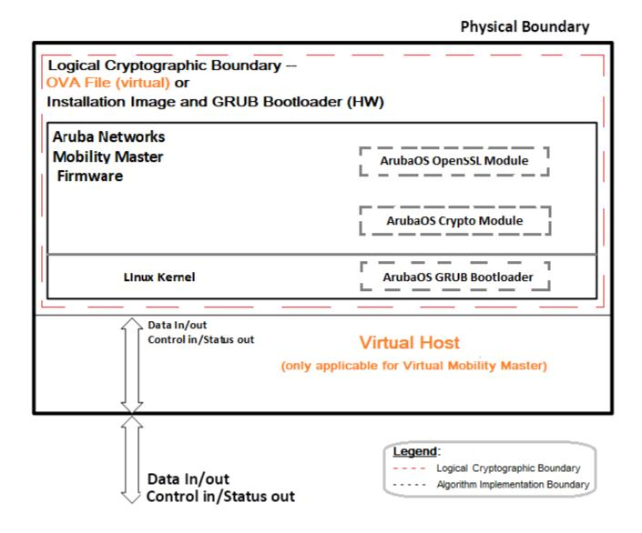
Figure 1: Functional Block Diagram of the System Component Stack
