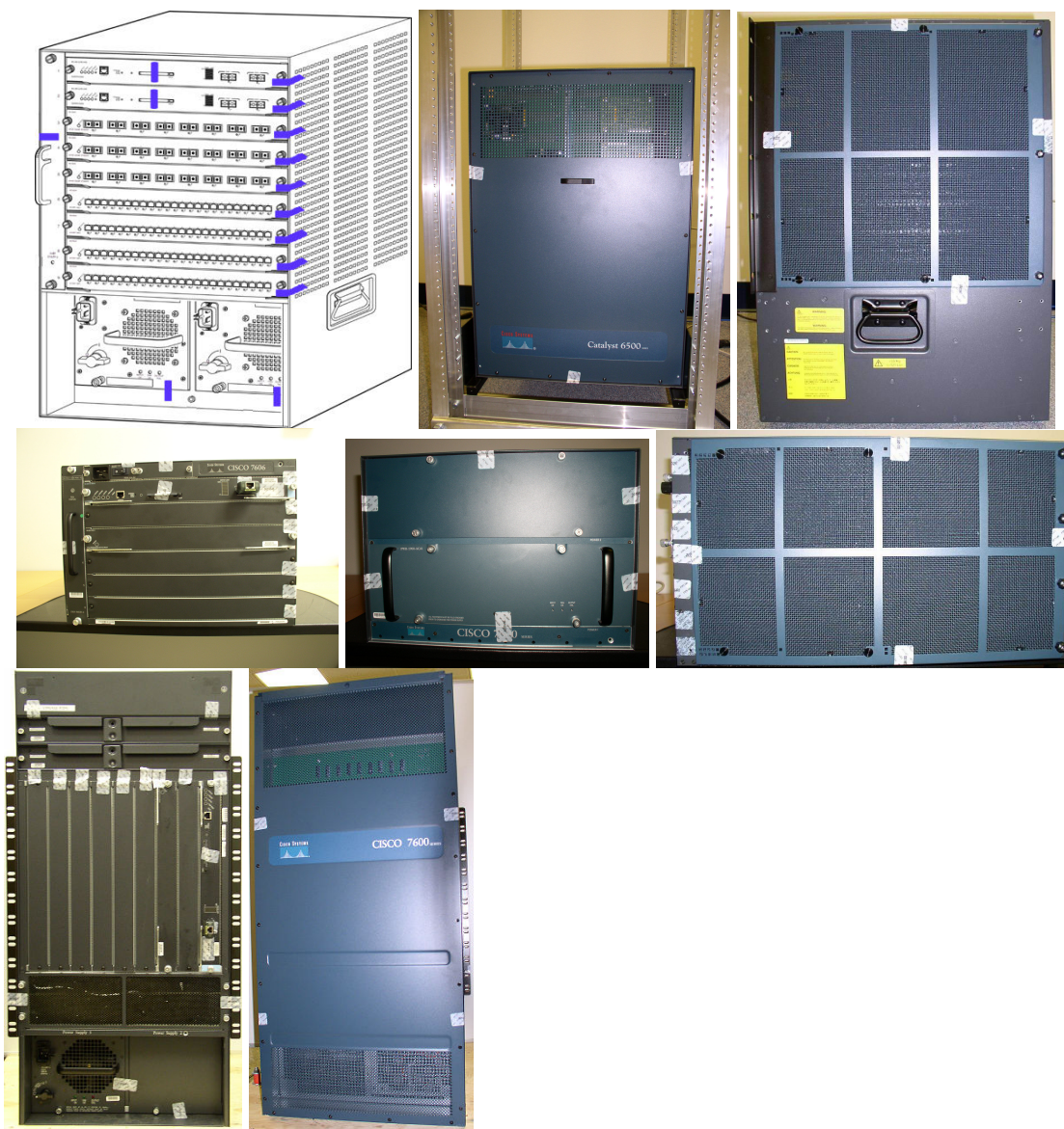
Figure 3 – 6509, 7606 and 7609 Tamper Evidence Label Placement
