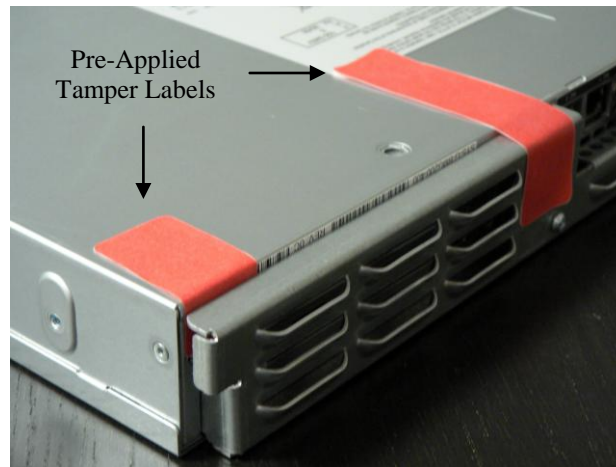
Figure 11 – B200 Rear Vent Label Placement
