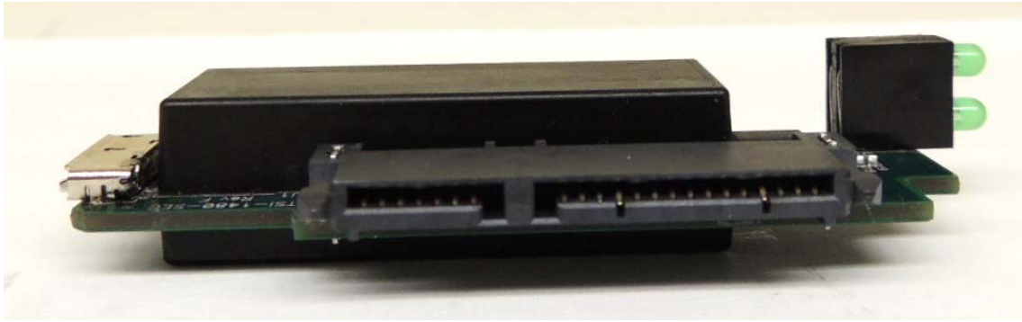
Figure 6 – KDH3000-CM – Left side view demonstrating the SATA port.
