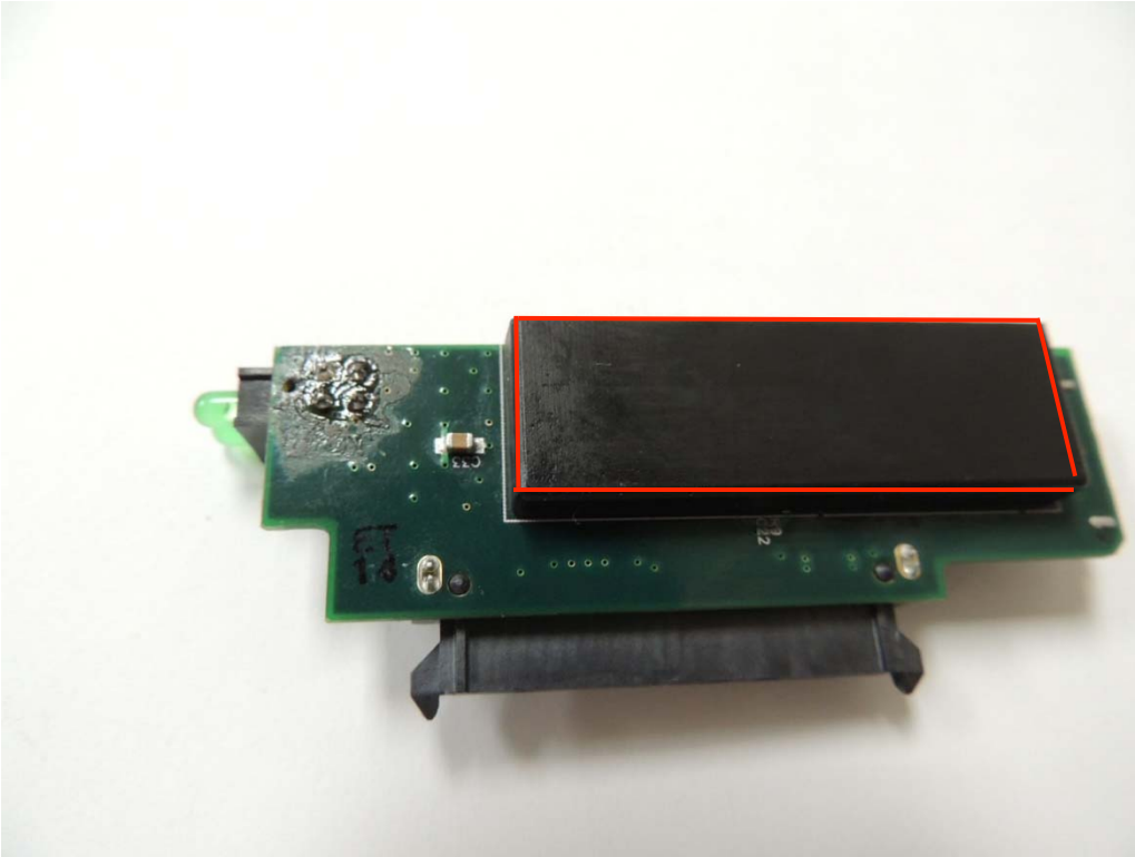
Figure 2 – KDH3000-CM – Bottom side view. The cryptographic boundary is defined by the area that the epoxy potting covers, which is outlined in red.
