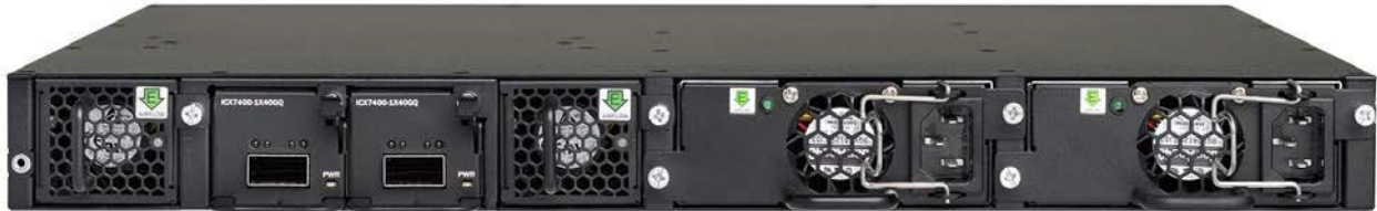
Figure 3 - Back side of ICX7450-48P with IPsec module inserted
