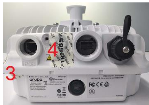
Figure 37 – Rear View of AP-377 with TELs
