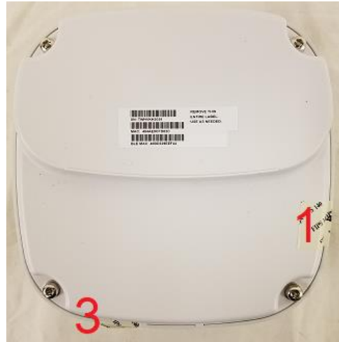
Figure 38 – Front View of AP-387 with TELs
