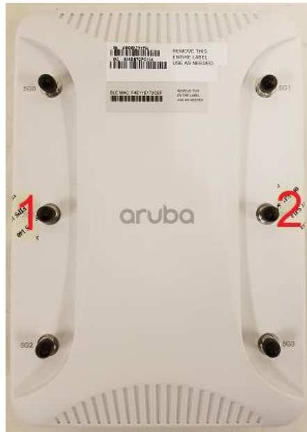
Figure 18 – Front View of AP-318 with TELs
