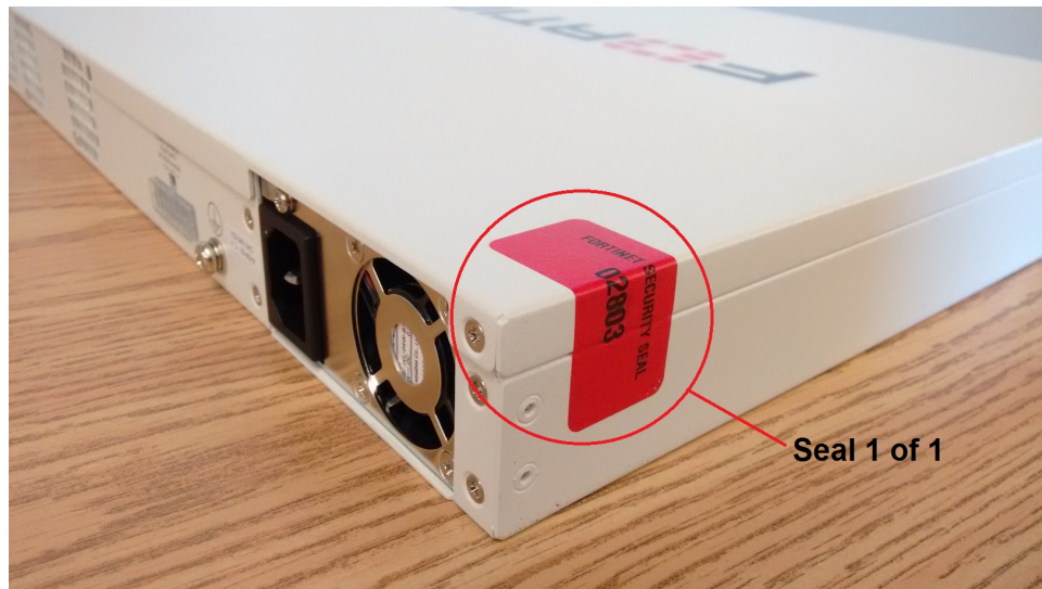
Figure 8: FortiGate-300D and 500D external enclosure seal, top, left side
