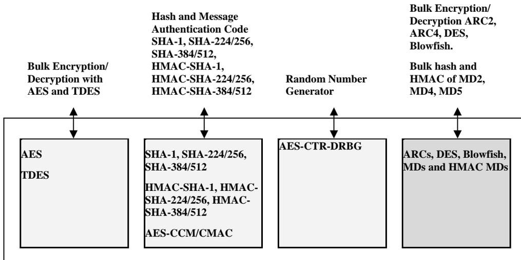
**Figure 2 – Logical Cryptographic Boundary**
