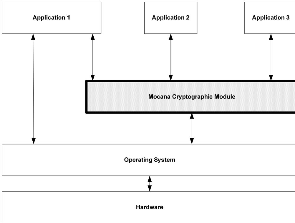
**Figure 1 – Cryptographic Module Interface Diagram**
