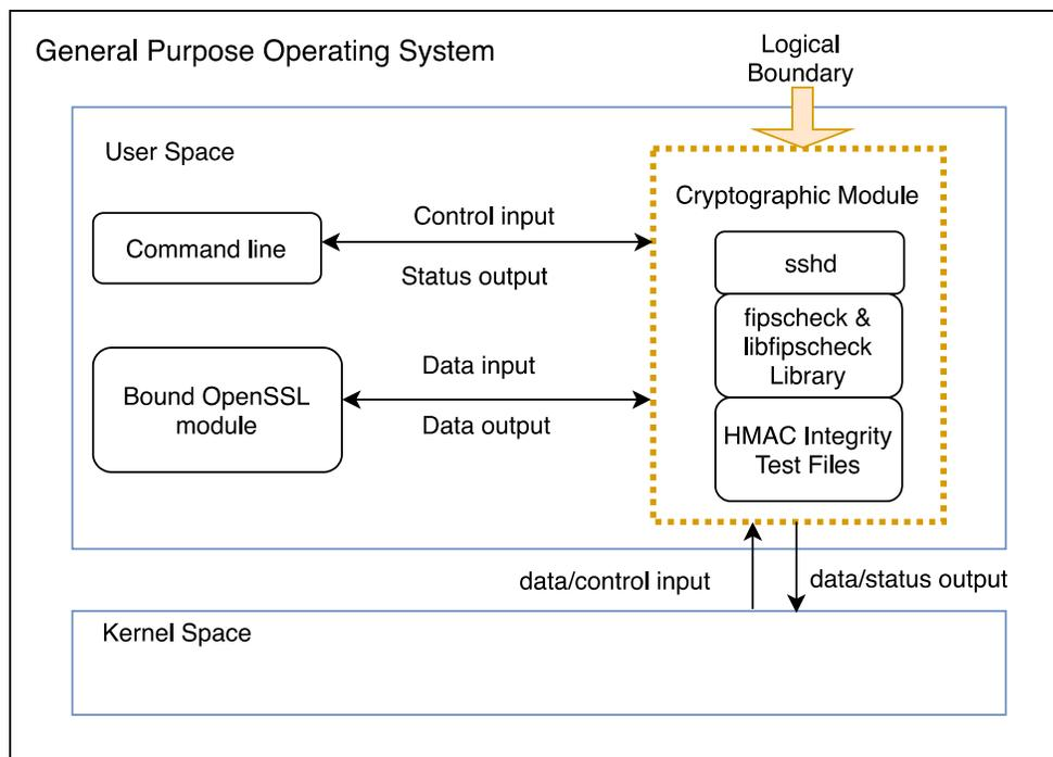
Figure 1: Logical cryptographic boundary.
