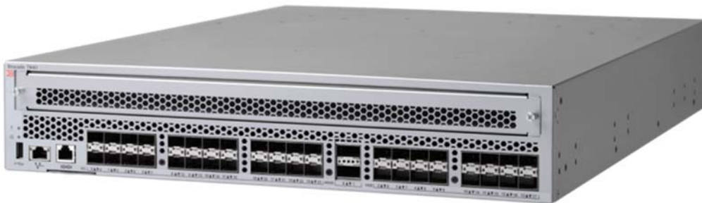
Figure 4 - Brocade 7840- Back and Top sides (showing XBR-FAN-80-R and XBR-1100WPSAC-R)
