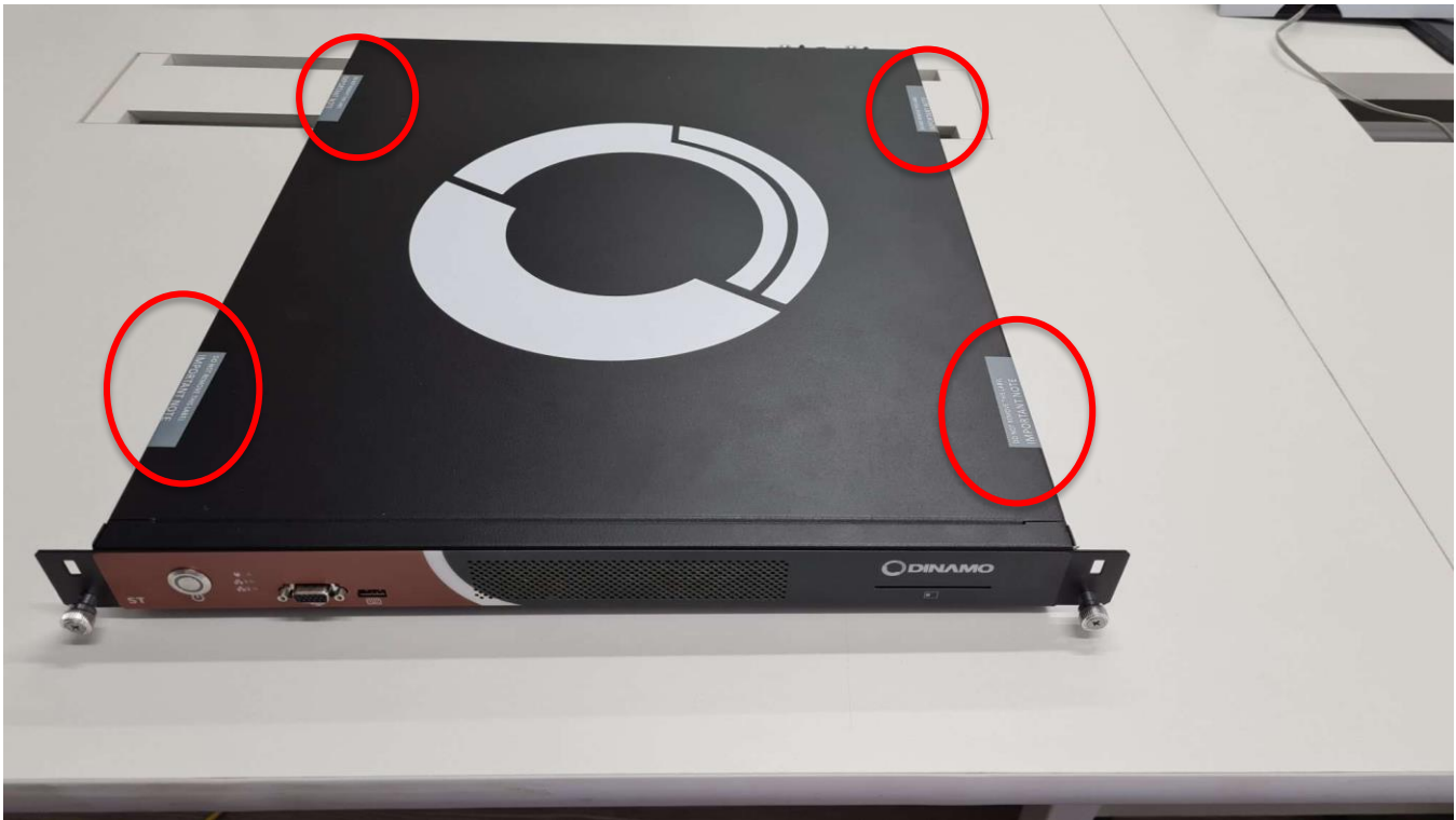
FIGURE 14 – Example of Tamper-Evident Seals Adjoining Top Cover to Base of Enclosure (DINAMO ST)
