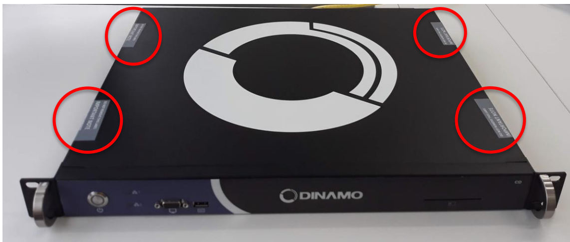
FIGURE 13 – Example of Tamper-Evident Seals Adjoining Top Cover to Base of Enclosure (DINAMO CD)
