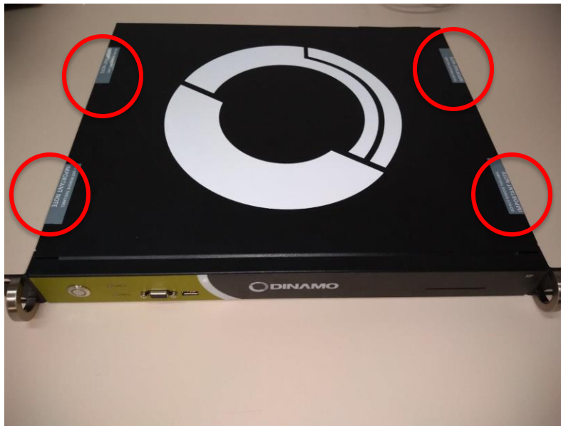
FIGURE 12 – Example of Tamper-Evident Seals Adjoining Top Cover to Base of Enclosure (DINAMO XP)
