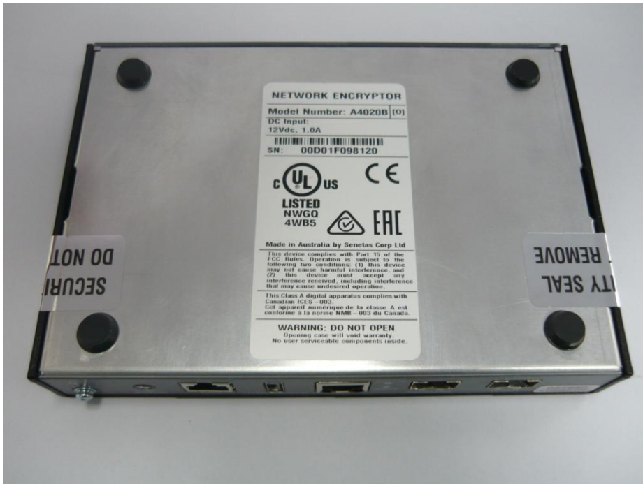
Figure 20 – CN4000 Series factory installed tamper seals
