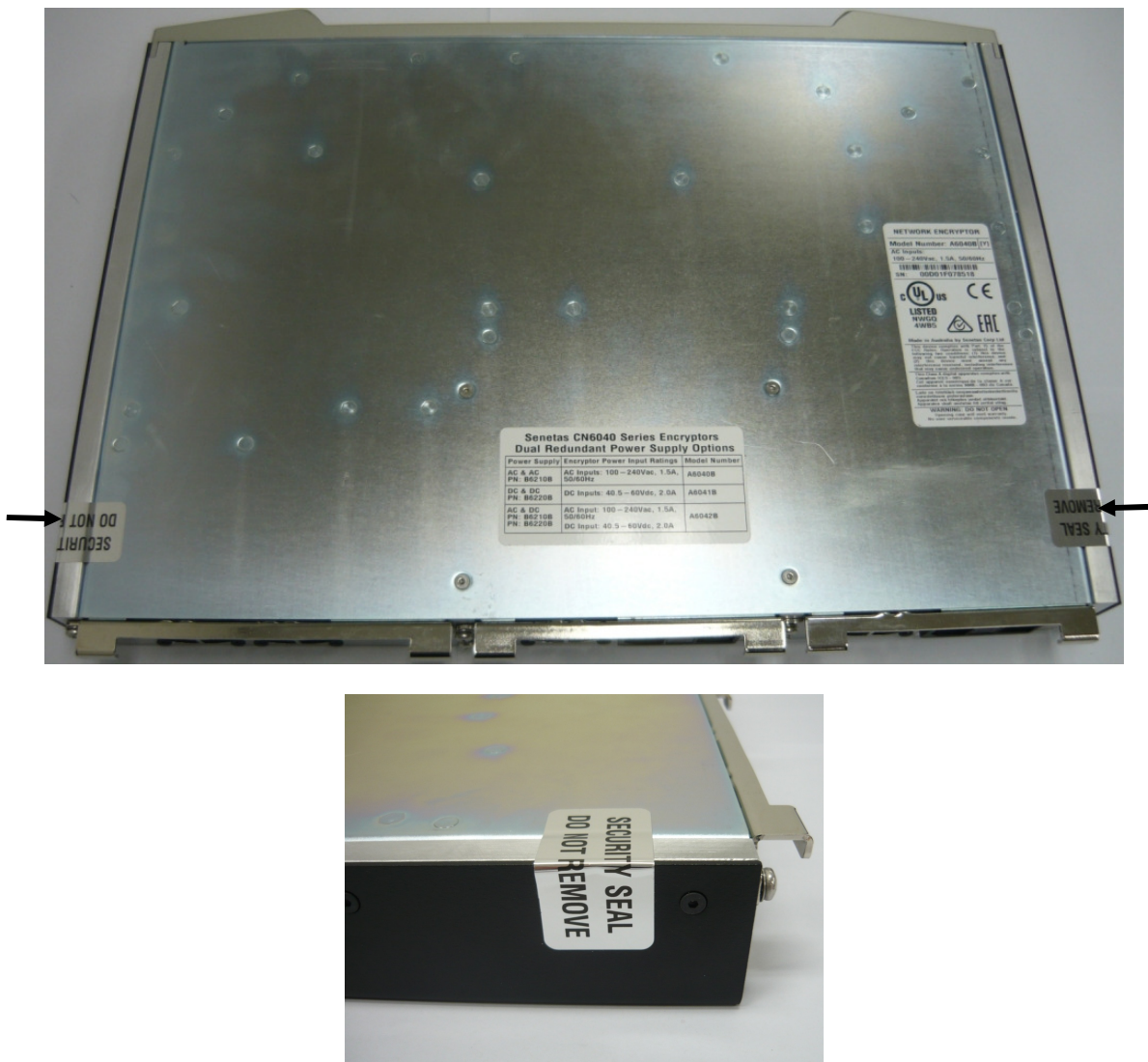
Figure 19 – CN6000 Series factory installed tamper seals
