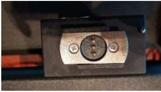
Figure 4 SC4200 showing the battery input.
