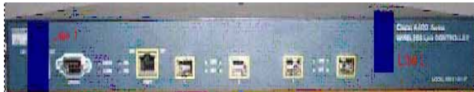
Figure 2 Placement of Tamper-evident Labels (Rear View)
