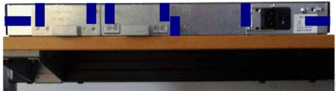
Figure 2 Placement of Tamper-evident Labels (Rear View)
