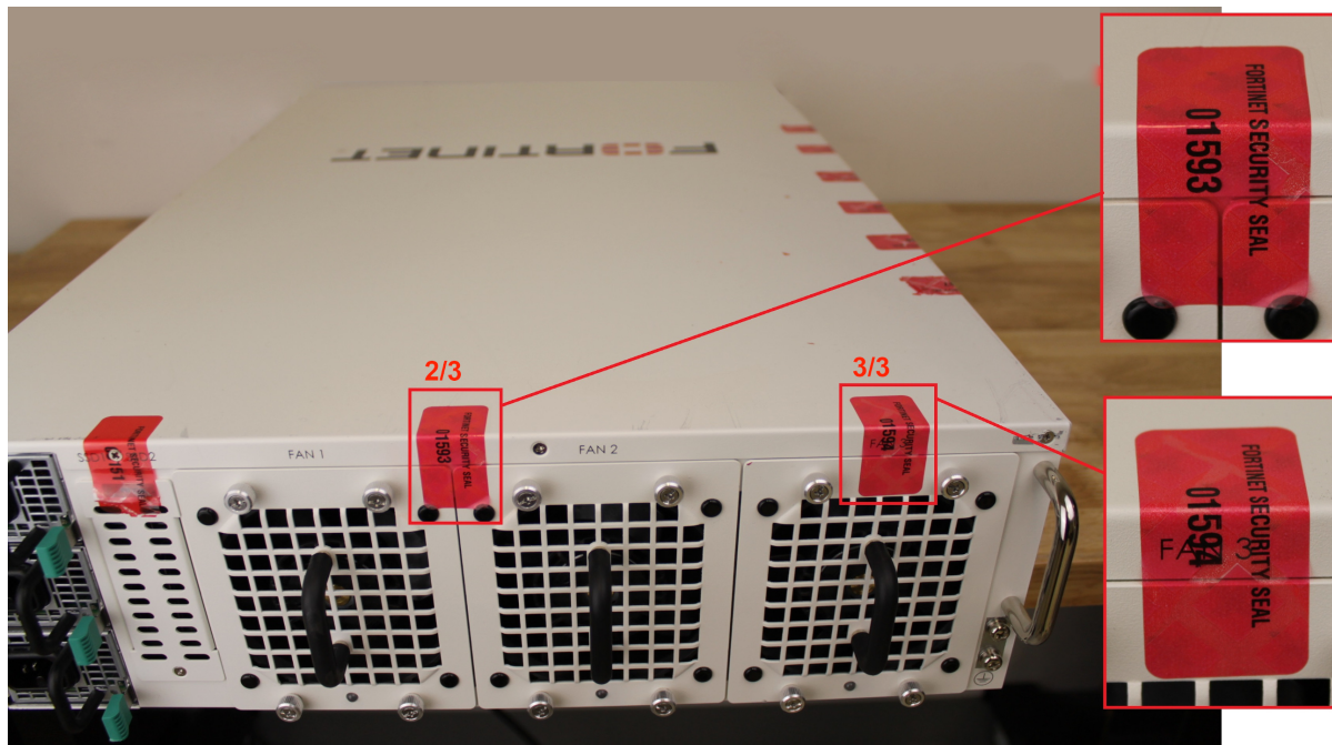
Figure 38 - FortiGate-6300F/6301F/6500F/6501F external enclosure seal 2 and 3, top, rear
