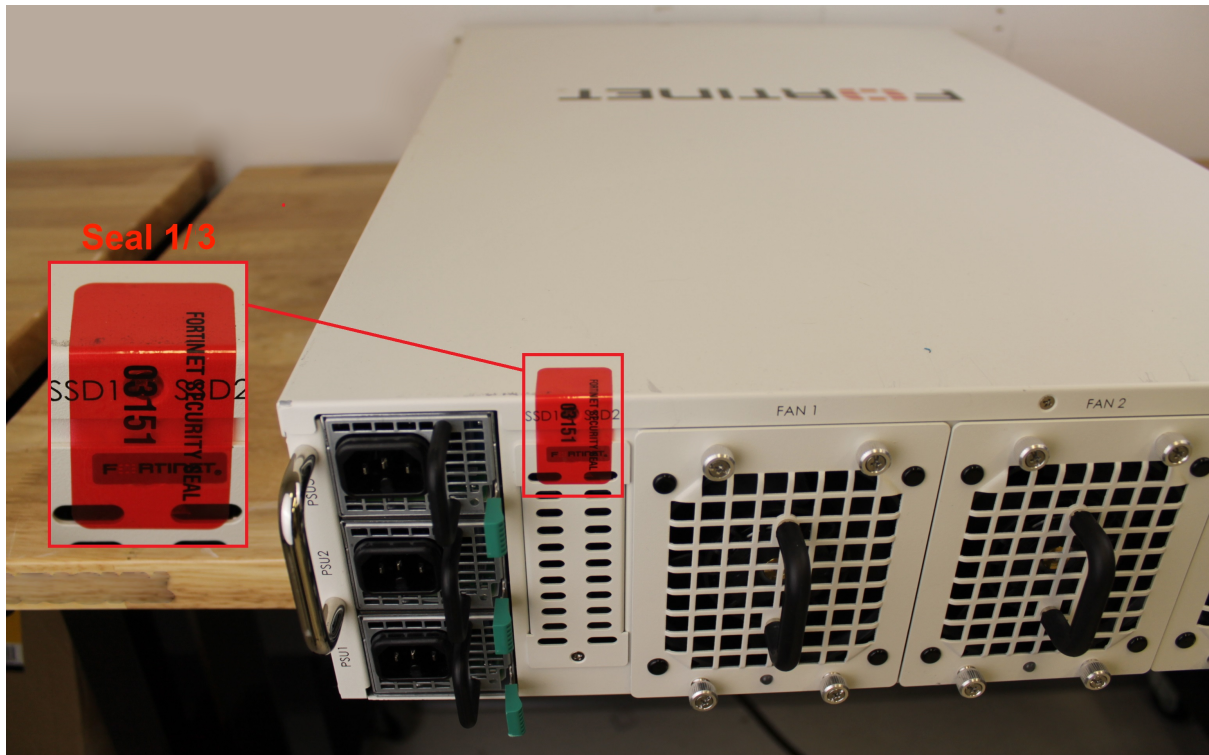
Figure 37 - FortiGate-6300F/6301F/6500F/6501F external enclosure seal 1, top, rear
