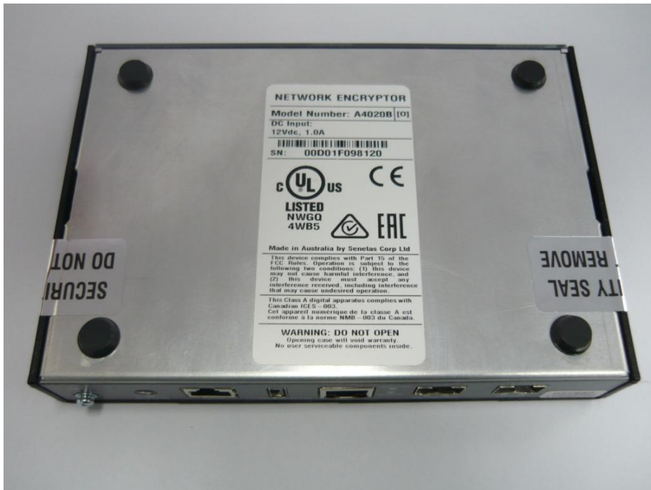
Figure 23 – CN4000 Series factory installed tamper seals
