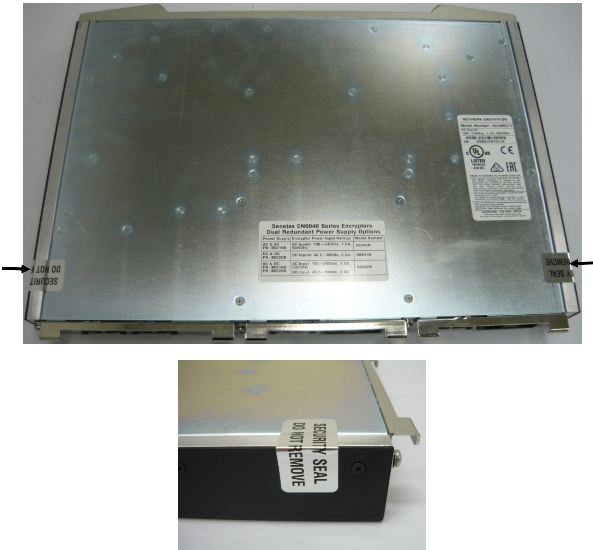
Figure 22 – CN6000 Series factory installed tamper seals
