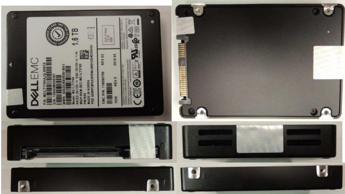
Exhibit 14 – Specification of the Samsung SAS 12G TCG Enterprise SSC SEDs PM1643/PM1645 Series, MZIL1T6HAJQ-000C9, Cryptographic Boundary (From top to bottom – Left to right: top side, bottom side, front side, back side, left side, and right side).
