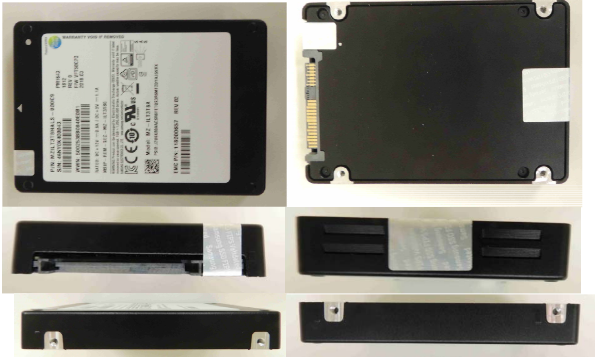
Exhibit 6 – Specification of the Samsung SAS 12G TCG Enterprise SSC SEDs PM1643/PM1645 Series, MZIL3T8HALS-000C9, Cryptographic Boundary (From top to bottom – Left to right: top side, bottom side, front side, back side, left side, and right side).
