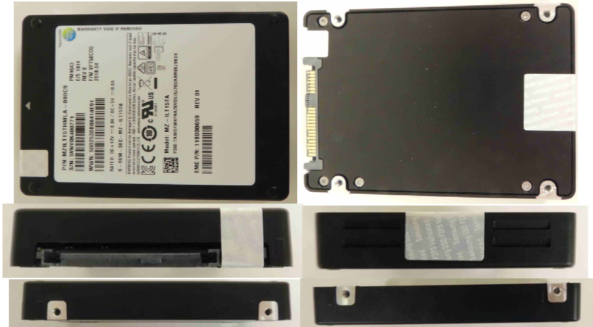
Exhibit 10 – Specification of the Samsung SAS 12G TCG Enterprise SSC SEDs PM1643/PM1645 Series, MZILT15THMLA-000C9, Cryptographic Boundary (From top to bottom – Left to right: top side, bottom side, front side, back side, left side, and right side).
