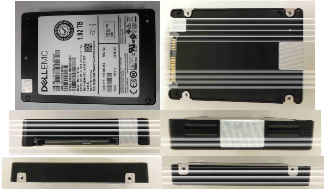
Exhibit 5 – Specification of the Samsung SAS 12G TCG Enterprise SSC SEDs PM1643/PM1645 Series, MZIL1T9HAJQ-00AC9, Cryptographic Boundary (From top to bottom – Left to right: top side, bottom side, front side, back side, left side, and right side).
