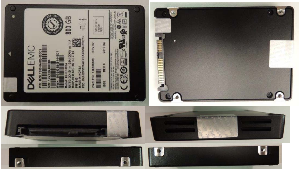
Exhibit 13 – Specification of the Samsung SAS 12G TCG Enterprise SSC SEDs PM1643/PM1645 Series, MZIL7800HAHQ-000C9, Cryptographic Boundary (From top to bottom – Left to right: top side, bottom side, front side, back side, left side, and right side).
