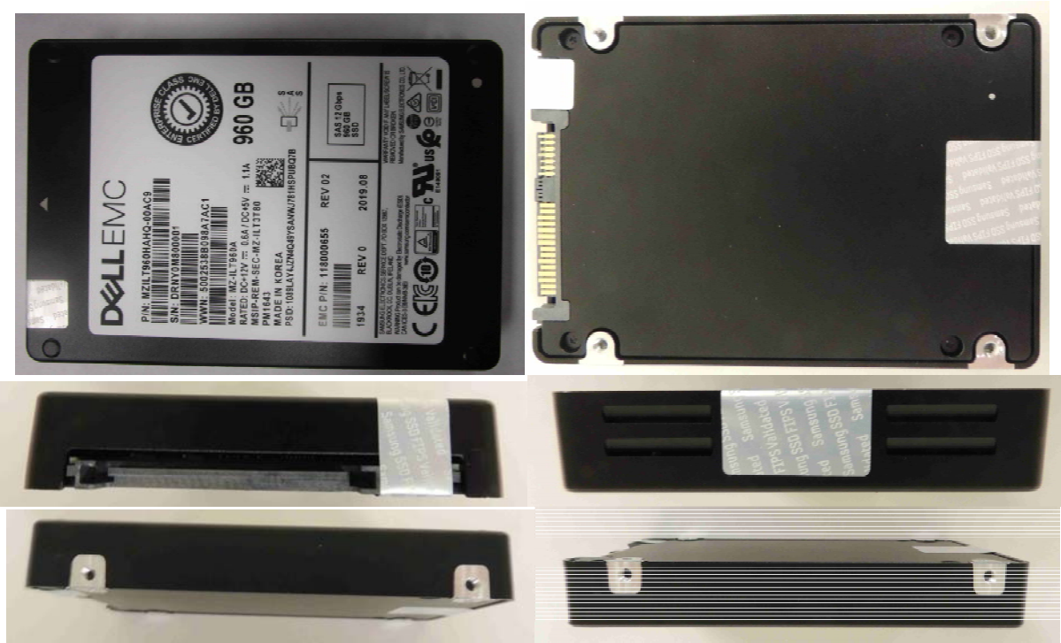
Exhibit 3 – Specification of the Samsung SAS 12G TCG Enterprise SSC SEDs PM1643/PM1645 Series, MZIL1960HAHQ-00AC9, Cryptographic Boundary (From top to bottom – Left to right: top side, bottom side, front side, back side, left side, and right side).
