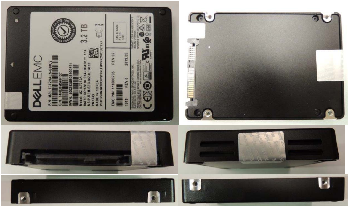
Exhibit 15 – Specification of the Samsung SAS 12G TCG Enterprise SSC SEDs PM1643/PM1645 Series, MZILT3T2HALS-000C9, Cryptographic Boundary (From top to bottom – Left to right: top side, bottom side, front side, back side, left side, and right side).
