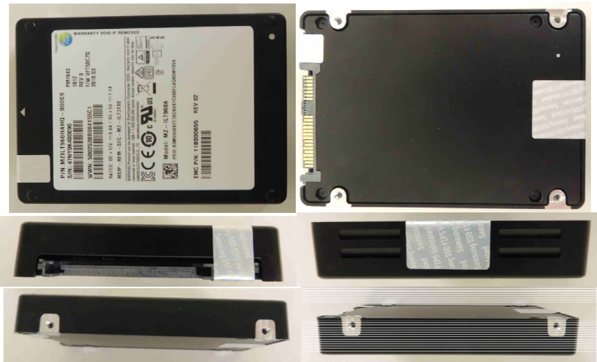
Exhibit 2 – Specification of the Samsung SAS 12G TCG Enterprise SSC SEDs PM1643/PM1645 Series, MZILT960HAHQ-000C9, Cryptographic Boundary (From top to bottom – Left to right: top side, bottom side, front side, back side, left side, and right side).
