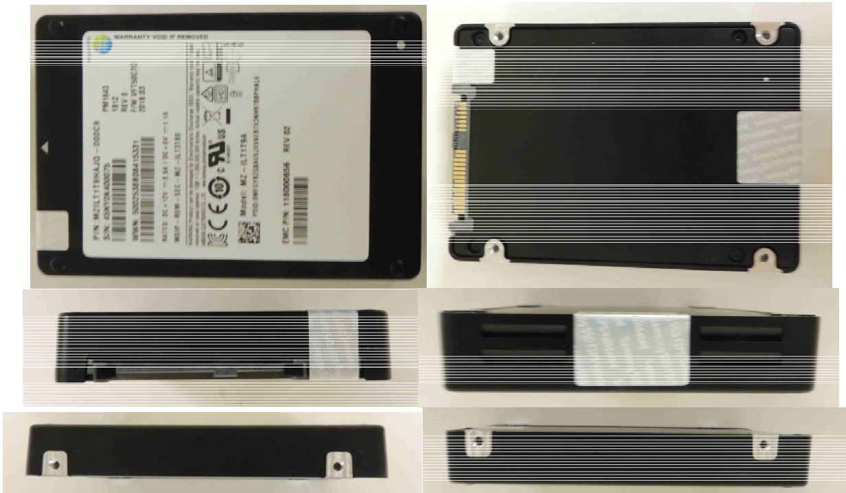
Exhibit 4 – Specification of the Samsung SAS 12G TCG Enterprise SSC SEDs PM1643/PM1645 Series, MZILT1T9HAJQ-000C9, Cryptographic Boundary (From top to bottom – Left to right: top side, bottom side, front side, back side, left side, and right side).
