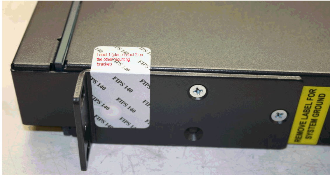
Figure 2 Placement of Tamper-evident Labels on Mounting Brackets
