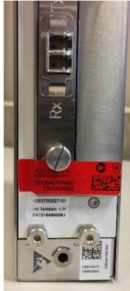
Figure 31 shows the location of the tamper-evident wire seal, ADVA part number 1013700032-01. The wire is threaded through the cross-drilled top mounting screws that secure the card in the 9U shelf.
