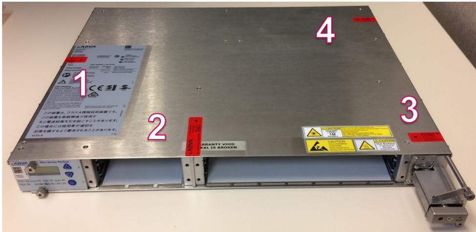
Figure 24 Seal Locations on Bottom of 1U Shelf with Rear Power Access
