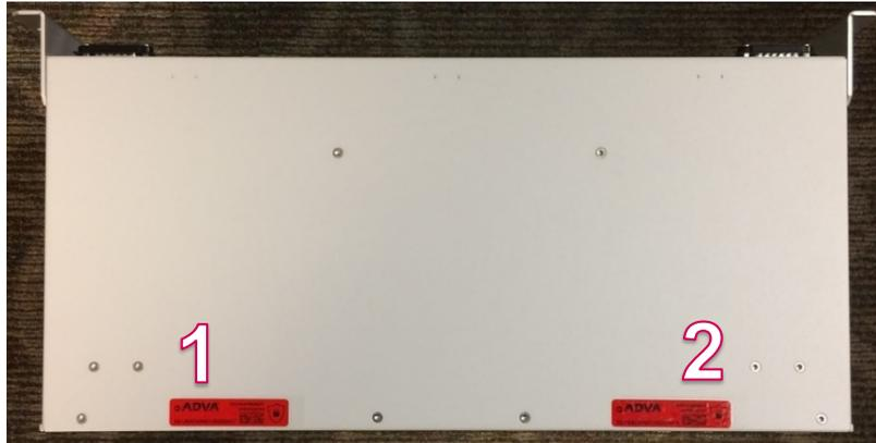
Two (2) seal locations on the rear of the shelf are marked in Figure 29:
