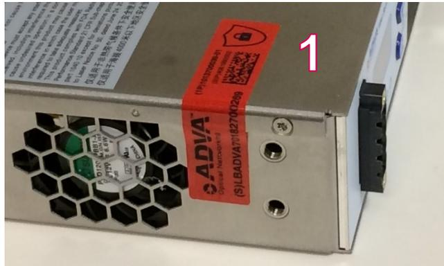
See Figure 20 for a close-up view of seal #2's location on the 1U shelf with front DC power access. The seal must be placed on the top cover near the center of the front panel area to cover the "Guarantee Void" label, which in turn covers the screw that holds the chassis card slot separator.
