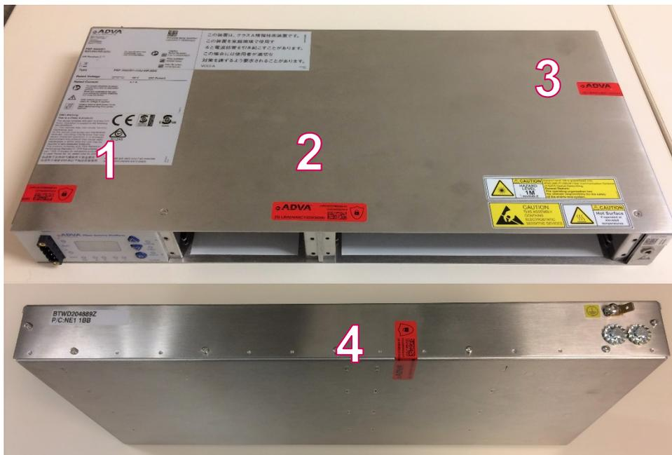
See Figure 19 for a close-up view of seal #1's location on the 1U shelf with front DC power access. The seal must be placed on the top cover at the front left edge and must wrap onto the left side.
