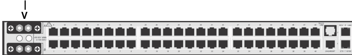
Figure 3 LX-4000T Series Typical Dual DC Rear Panel View (48 Port)
