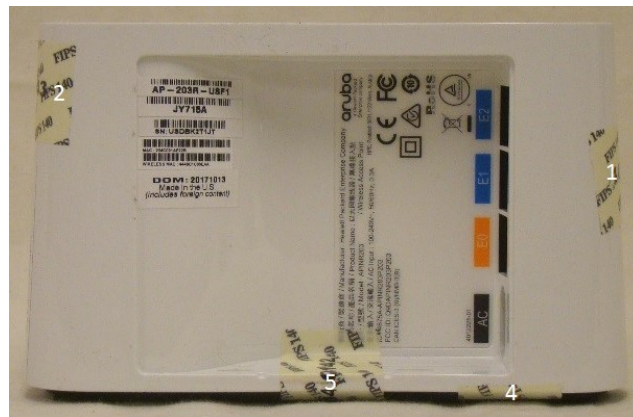
Figure 11 – Back View of AP-203R with TELs
