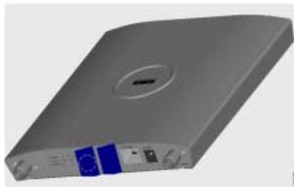
Figure 7 Placement of Tamper-evident Labels for the AP1242AG (Front View)
