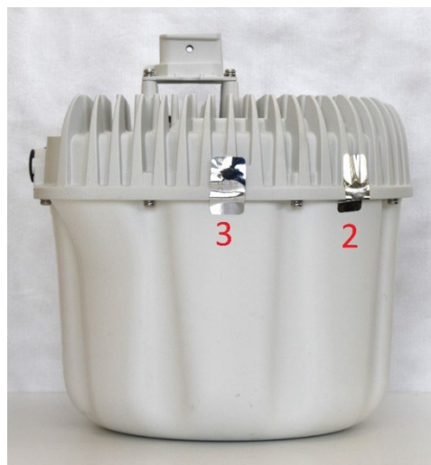
Figure 37 – Left Side View of AP-585 with TELs
