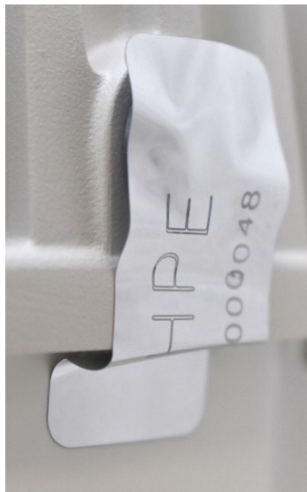
Figure 31 – Placement of TEL 3 on AP-580 Series APs
