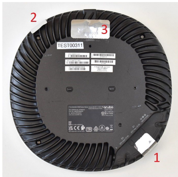
Figure 42 – Bottom View of Aruba AP-635 with TELs
