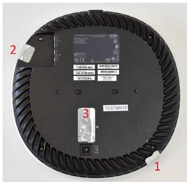
Figure 44 – Bottom View of Aruba AP-655 with TELs
