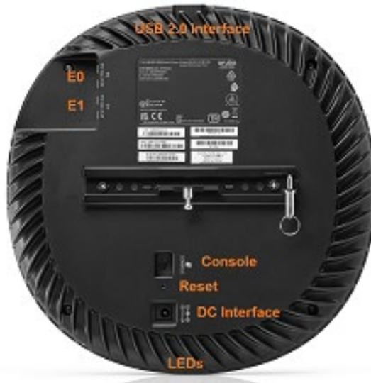
Figure 23 - AP-650 Series Campus Access Point – Interfaces
