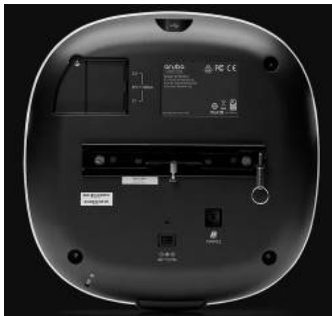
Figure 7 - AP-534 Campus Access Point – Back
