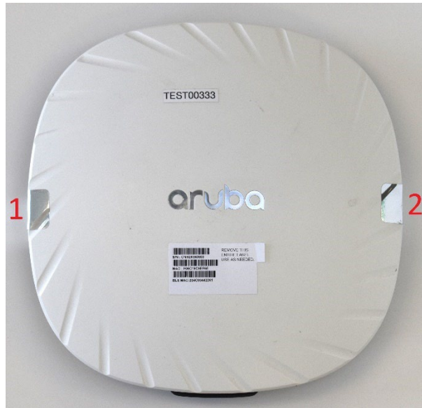
Figure 28 – Top View of AP-535 with TELs
