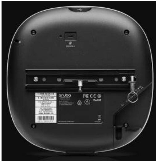
Figure 4 - AP-515 Campus Access Point – Back
