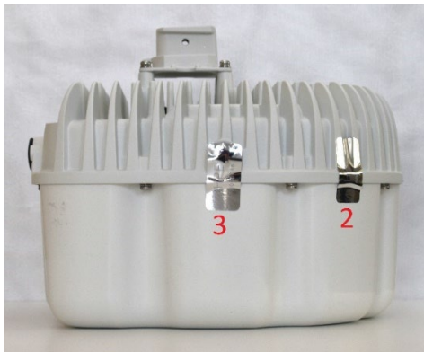
Figure 34 – Left Side View of AP-584 with TELs
