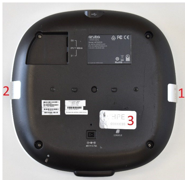
Figure 29 – Bottom View of Aruba AP-535 with TELs
