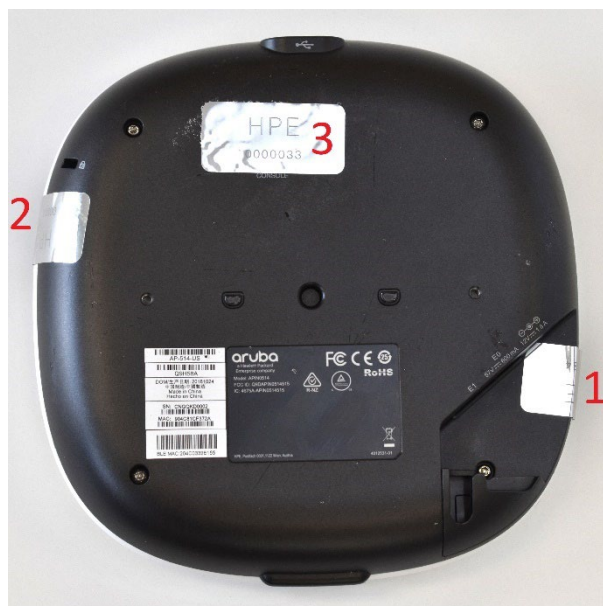
Figure 27 – Bottom View of Aruba AP-514 with TELs
