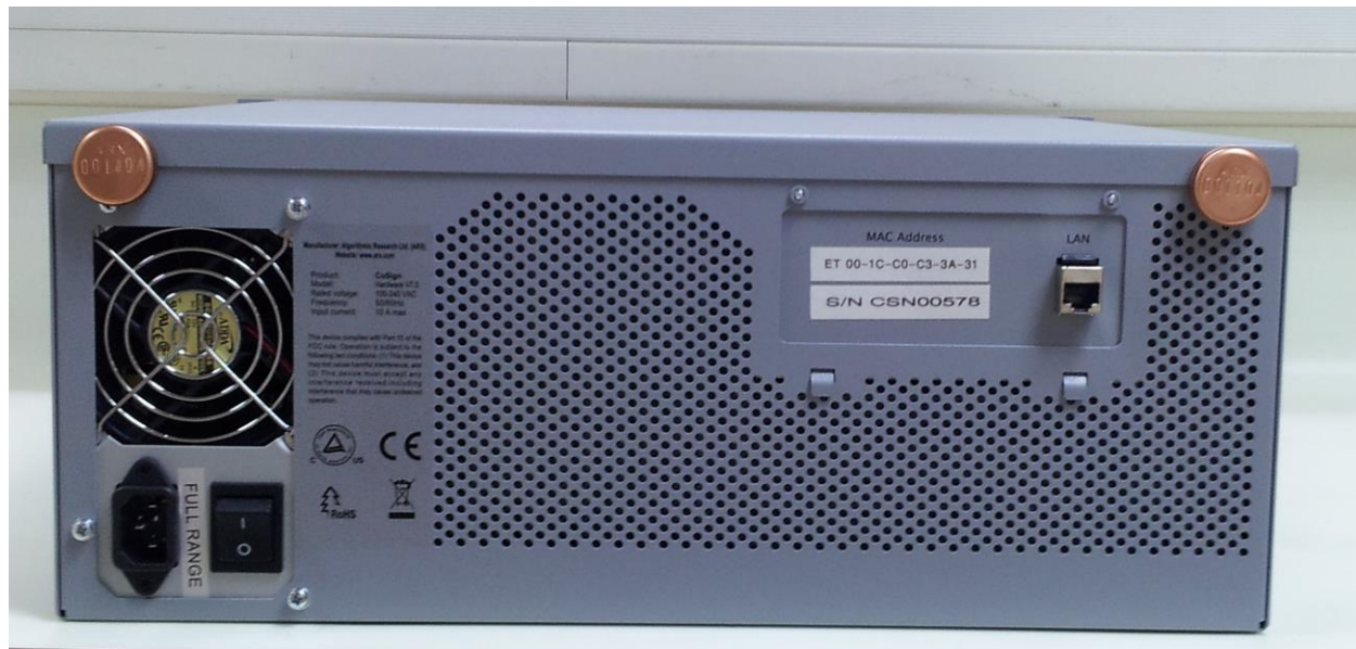
Figure 4 - Tamper Evident cans – DocuSign Signature Appliance - Hardware version 7.0
