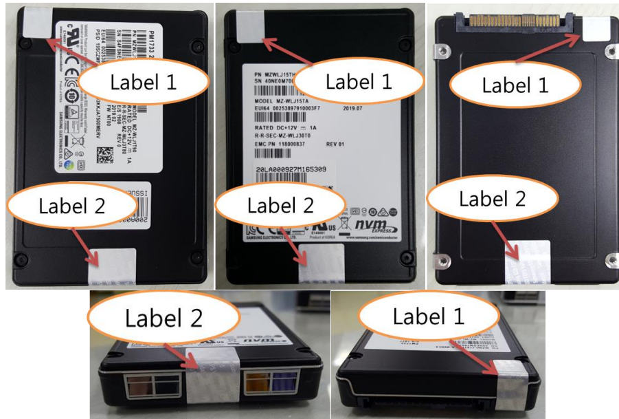
Exhibit 16 – Tamper Evident Label Placement
