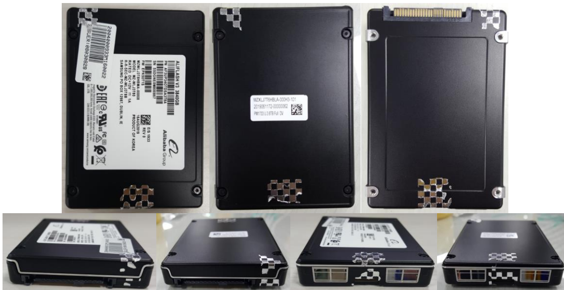
Exhibit 17 – Example of Signs of Tamper
