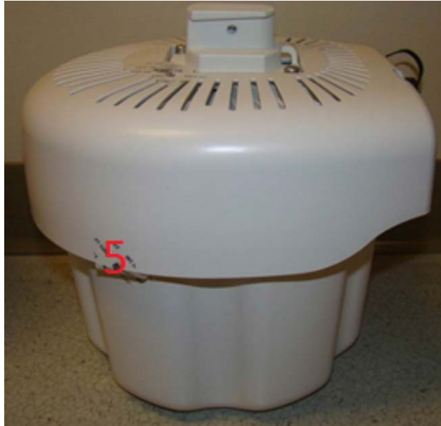
Figure 16 – Right Side View of AP-275 with TELs
