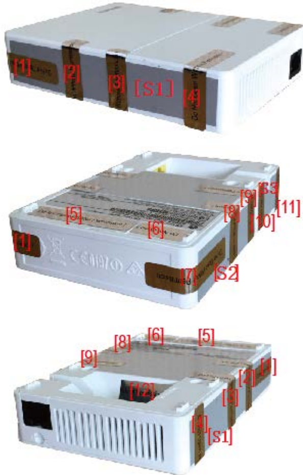
Figures 5-3 R250D tamper seal placement
