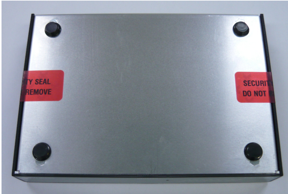
Figure 17 – CN4010 Factory installed tamper seals
