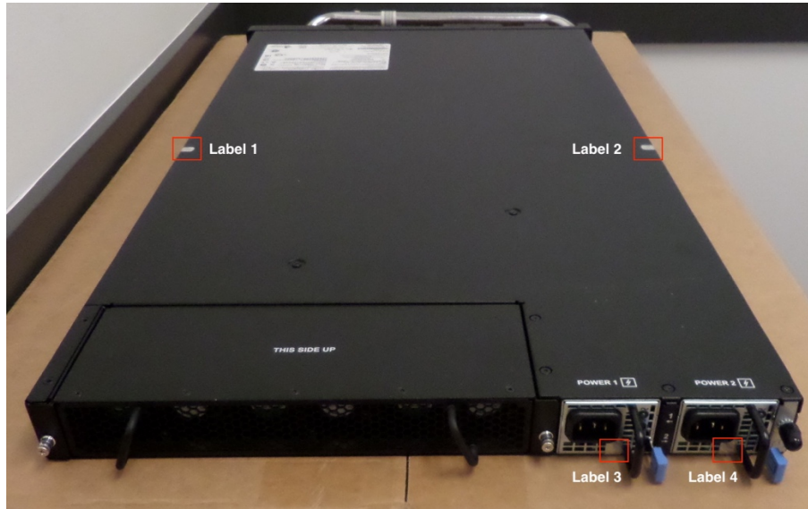
Figure 17 - BIG-IP i7820-DF (4 tamper labels shown)
