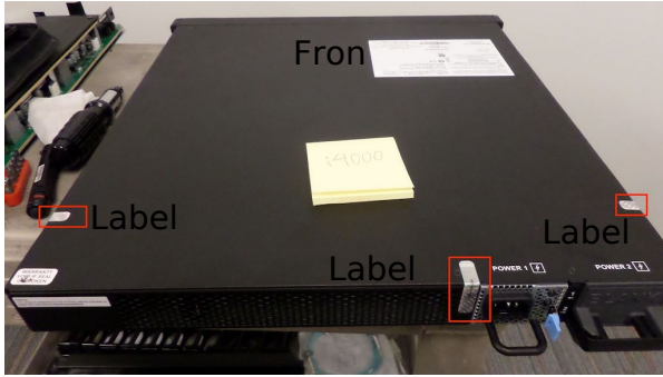
Figure 13 - BIG-IP i4000 (3 of 3 tamper labels)
