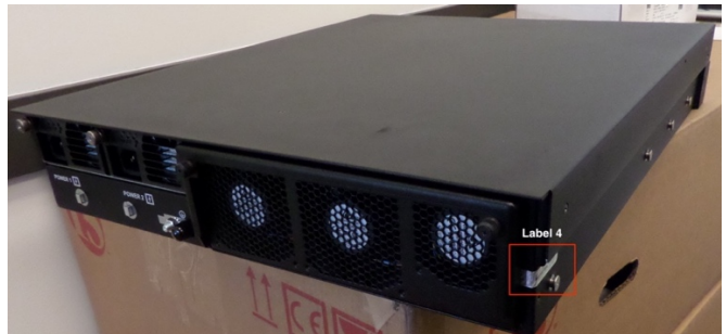
Figure 23 - BIG-IP 7200v-F (5 tamper labels shown)
