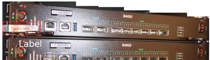
Figure 29 - VIPRION B4450 front (1 of 5 tamper labels shown)
