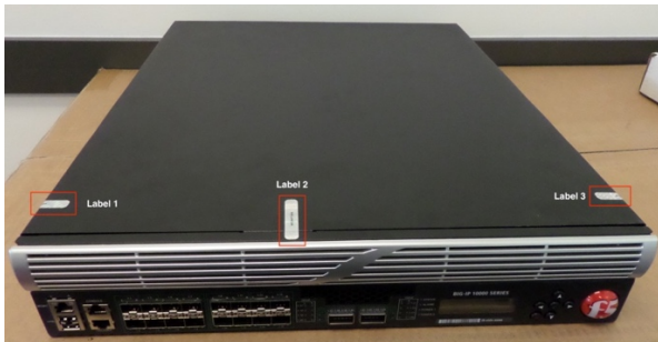
Figure 23 - BIG-IP 7200v-F (5 tamper labels shown)
