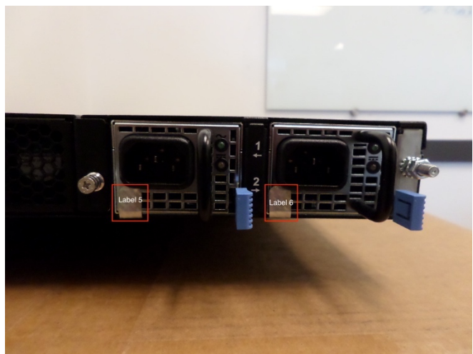
Figure 19 - BIG-IP i10800 / i11800-DS (tamper label 5 & 6)
