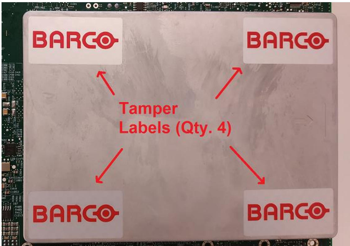
Picture 3 – Barco ICMP security enclosure tamper evident labels
