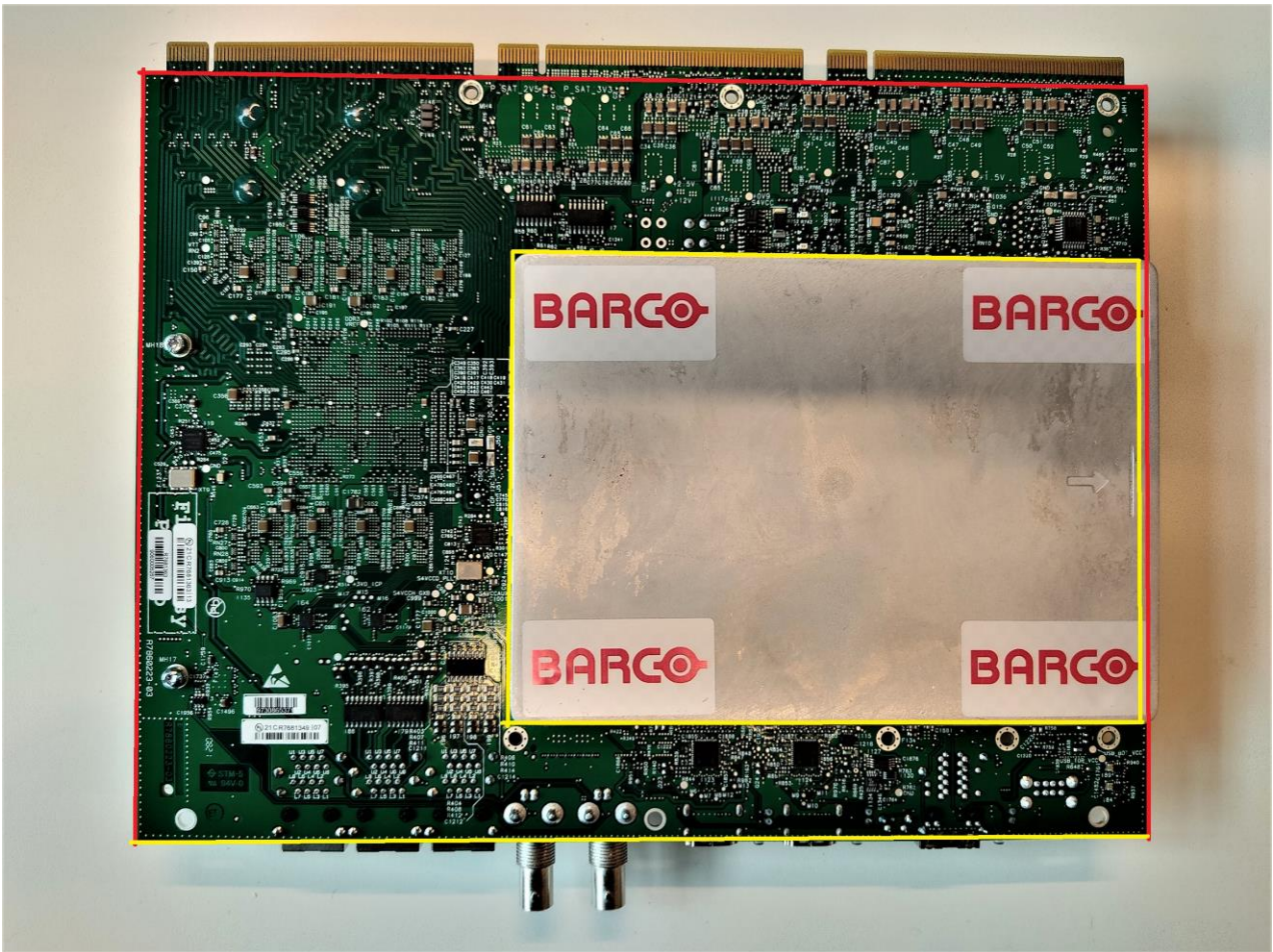
Picture 2 – Barco ICMP R7681360-09 main board bottom view
