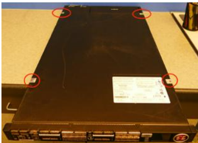
Figure 9 – Tamper labels on r10900, r10920-DF
