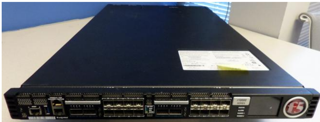
Figure 5 – r10900, r10920-DF front view (same chassis for the two test platforms)
