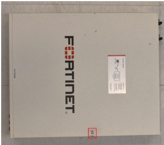
Figure 18: FG-3000F & 3001F Seal Placement
