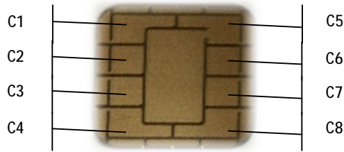
Figure 5: ISO 7816 Interface Contact Pad Designations and Locations
