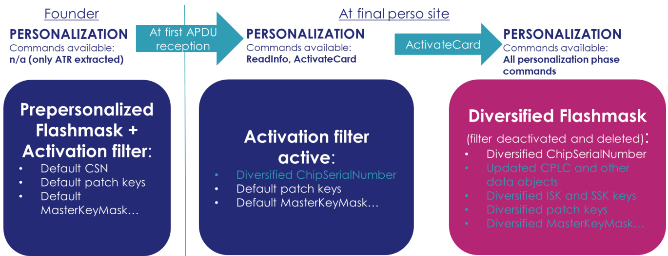
Figure 4: Delivery flow with the diversification filter mechanism
